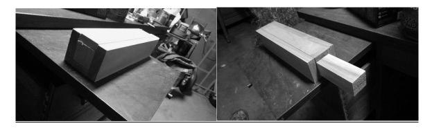
**Step 4:** Using the c-clamps, secure the outside boards together to make sure that they don't move when they are screwed together. (See picture below)
