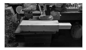
\* Note: The screw placement pattern that I used above is at the following measurements starting at the top of the stool: ½", ½", 7½", and 11½".
