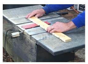
Next cut the ¼" plywood into 2" by 5.5" rectangles. You need 7 of these. These will be the dividers at the bottom. Place them in the slits on the bottom piece of the board. Use glue to secure them, if necessary or desired.
