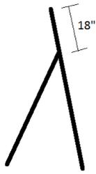
To stabilize the frame, use two pieces of 16-18" long chain. Use screws to attach it to the lower horizontal bar on the front legs, about 5 inches in from the outer edge. The other end will attach on the back side of the back legs. Putting it on the back side allows the stand to fold up without pinching the chain.
