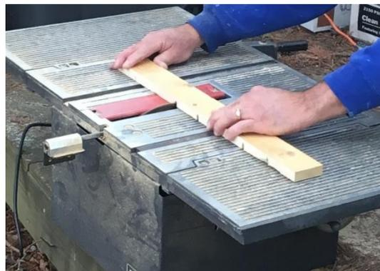
Next cut the  $\frac{1}{4}$ " plywood into 2" by 5.5" rectangles. You need 7 of these. These will be the dividers at the bottom. Place them in the slits on the bottom piece of the board. Use glue to secure them, if necessary or desired.
