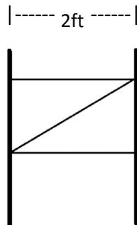
Cut two pieces of 2x4 to be 48in each. These will be the back legs. Cut one piece to be 28in. Use screws to connect the two longer pieces with the 28in piece at the bottom to make a "U" shape. Attach wheels or castors on the bottom of the 28in piece.
