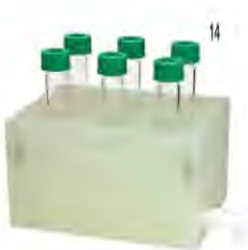
Figure 1: SPPS Vessels with Billboard. Containers used for the solid phase peptide synthesis in the billboard with a drain.
