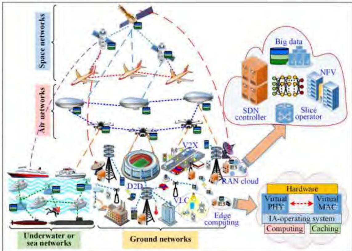
The typical architecture of 6G network (ISAGUN). V2X: vehicle to everything; VLC: visible light communication; RAN: radio access networks; SDN: software-defined networking; NFV: network function virtualization; PHY: physical layer; MAC: medium access control (Yang et al., 2019).
